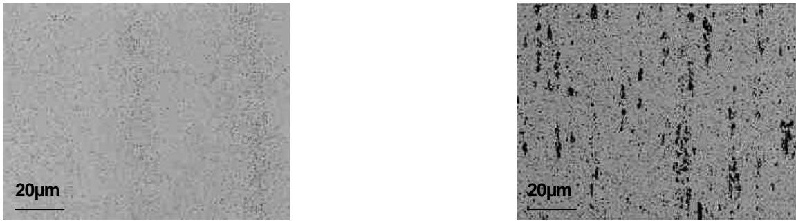
Figure 2 : Banding carbide structure of XD15NW and X105CrMo17
