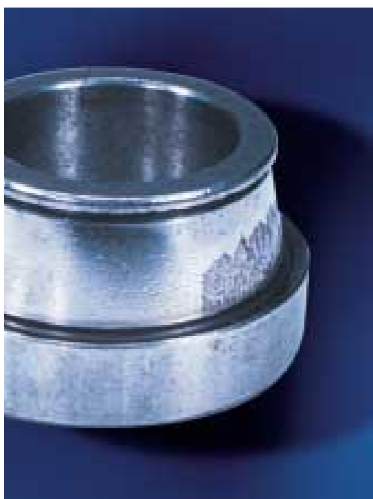
Cone spalling due to misalignment
