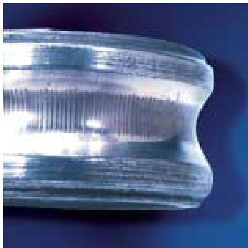
Electric current through the rotating inner ring
