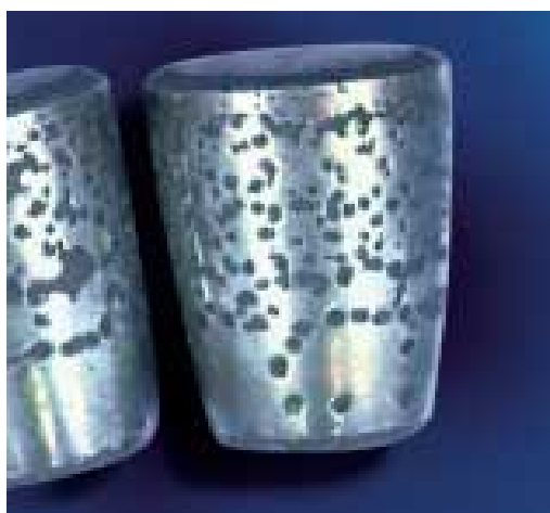
Pitting with dark bottoms on the rolling elements
