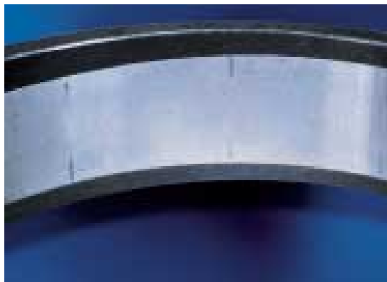
Material tears on the outer ring raceway
