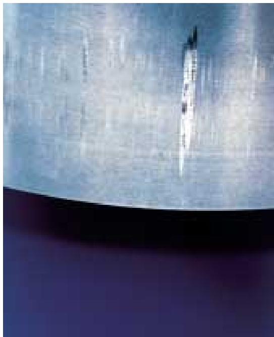
False brinelling on a roller bearing
