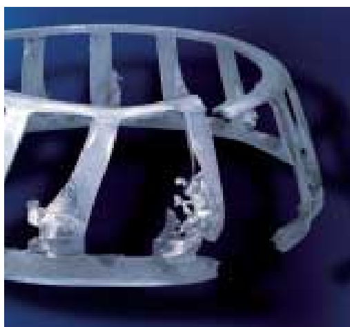
Cage damage due to incipient seizing
