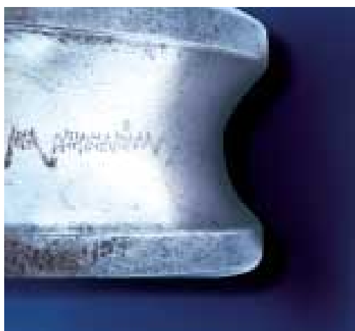
Electric arcing on the inner ring
