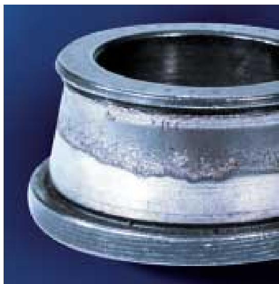
Cone spalling due to taper of the shaft or housing
