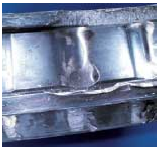
Seizing of a spherical roller bearing with roller imbedding and flange fracture
