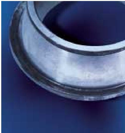
Damage to the flange due to excess preload
