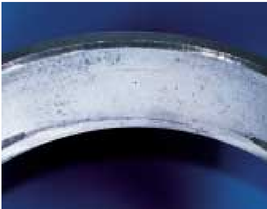
Damage caused by a geometric defect of the housing
