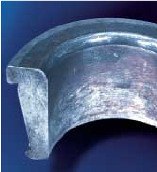
Contact corrosion in the bore and the abutment face
