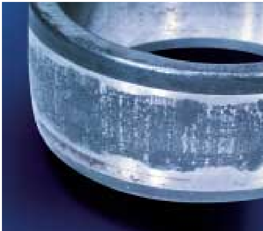
Corrosion when operating (liquid ingress)
