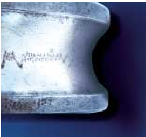
Electric arcing on the inner ring
