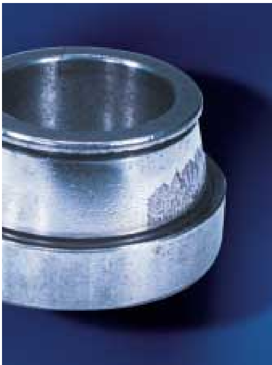
Cone spalling due to misalignment
