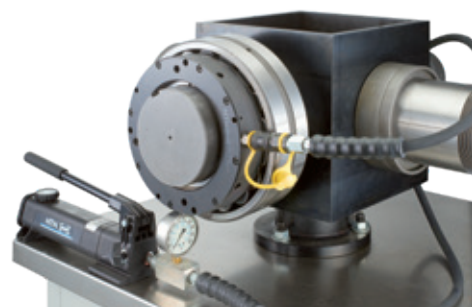
Extraction of the withdrawal sleeve with a hydraulic nut
