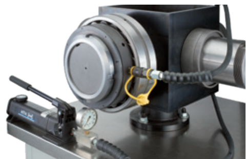
Mounting on withdrawal sleeve by indirect pushing of the hydraulic nut
