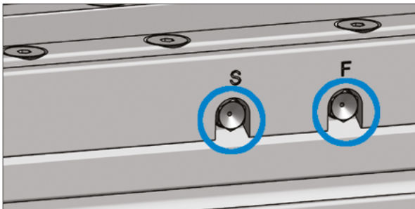
Figure 1.12 — Slider unit with laterally placed grease nipples
