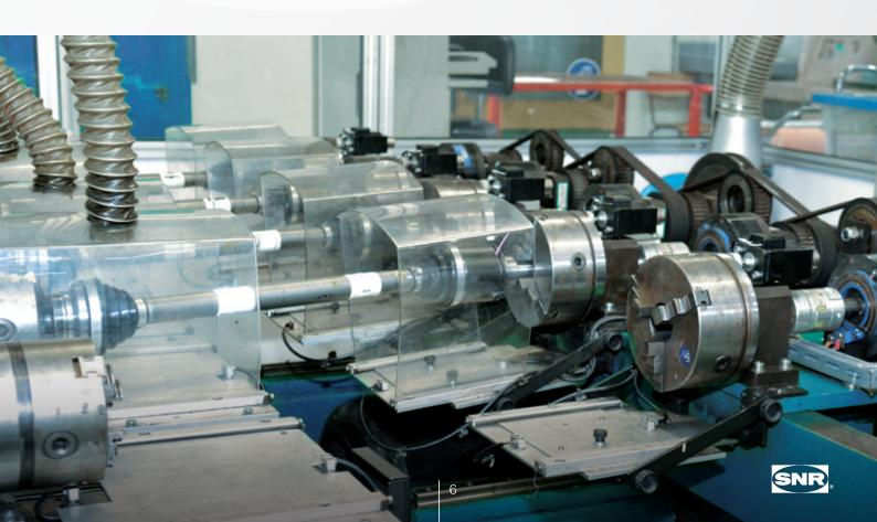
Lack of testing may put motorists at risk as a incorrectly manufactureed CVJ may fail with the loss of drive to the wheels, increasing the chances of the wheel breaking away from the vehicle.
