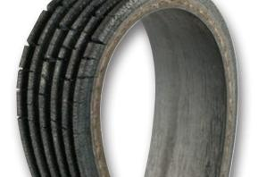
CAUSES • Over heating of the belt caused by friction. An over tightened belt causing it to stretch and crack. CAUSES • Too low or too high working temperature. • Ageing of the belt. Contact with a foreign element or a misalignment issue.
