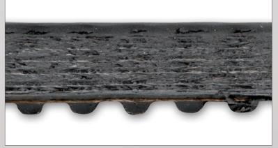
CAUSES • The belt slipping over the tensioner, due to low tension on the belt when in operation.
