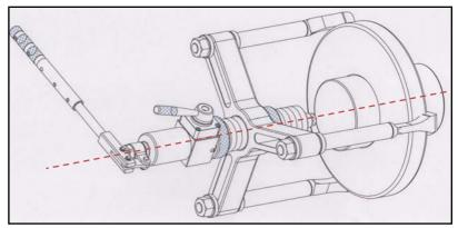
2. Move the adjusting ring 1 clear of the cross-head. Rotate the hydraulic cylinder to move it towards the point of support on the shaft moving back the adjusting ring 2 as required. Wrap the work with a protective blanket when ready to start pulling.
