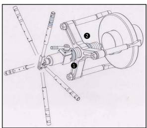
3. Once sure of correct puller alignment, switch the control valve knob to the "Advance" position and start to pump the handle to extend the piston until it touches the shaft centre. Ensure the jaws evenly grip around the part to be pulled. Continue pumping the handle until the object to be pulled is removed.
