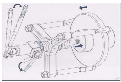
4. After the object has been removed, switch the control valve knob to the "Retract" position to fully retract the piston.
