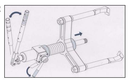
3. Securely connect the piston to the "connector" and postion the 3 arms evenly against the inner edge of the object. Adjust the position of the hydraulic cylinder moving the adjusting ring 1 as required. Ensure the adjusting ring 2 remains clear of the crosshead.
