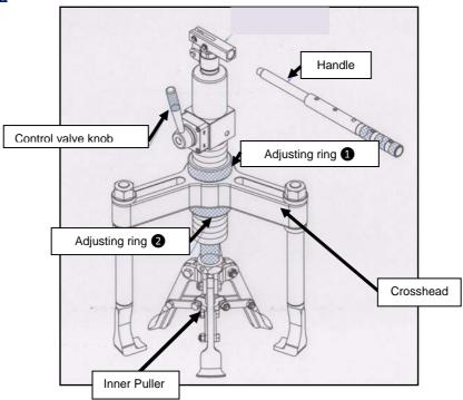
1. Insert the inner puller through the object and turn the hex nut in a clockwise direction to spread the arms until they grip firmly behind the inner edge of the object.
