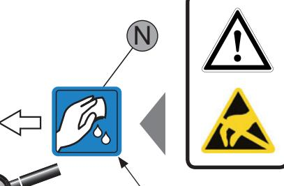
The enclosure is constructed from plastic. To prevent the risk of electrostatic sparking the plastic surface should only be cleaned with a damp cloth. Appropriate measures must be taken to prevent electrostatic discharge.
