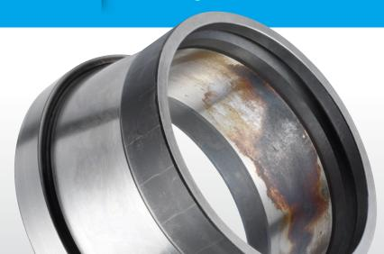
Bearings are a wearing part and will fail eventually. Despite being machined to very close tolerances from high-performance steel, bearings have a limited service life. Indeed, the loads applied to bearings will eventually result in fatigue failure of the material which limits the service life. However, on top of the fatigue failures, many other external factors to the bearings influence the life and can lead to premature failure.
