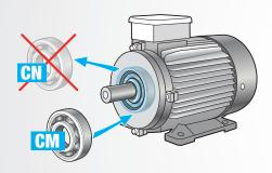
Replacing the **CN** clearance with the **CM** clearance **has no impact on mounting.**
