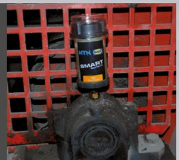
*Effective, precise, flexible lubrication for applications subject to wide variations in temperature or situated in explosive environments.*
