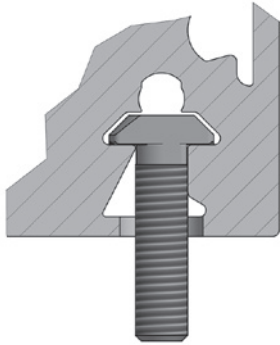
Figure 6.7 ___ Linear Axis AXF with hammer screws
