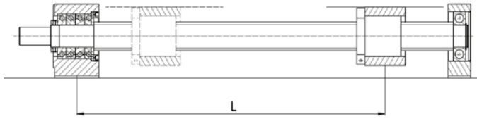
Figure 2.15 __ Bearing arrangement fixed - supported
