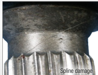
Fracture of cup stem
