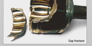
• Fracture of cup stem • Fracture of a connecting spline • Fracture of part of the cup Result: No longer transmits torque from the gearbox to the wheels
