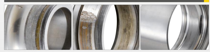
CAUSES Fatigue Incorrect installation • Incorrect geometry of a neighboring parts
