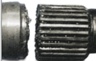
Fracture of connecting spline
