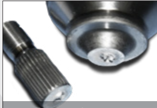
Fracture of cup stem
