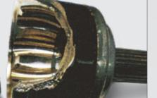
• Utilization of the product outside of the manufacturer's specifications • Incidental maneuver (example: impact start or running over kerb)
