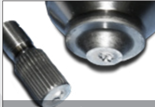
Fracture of cup stem
