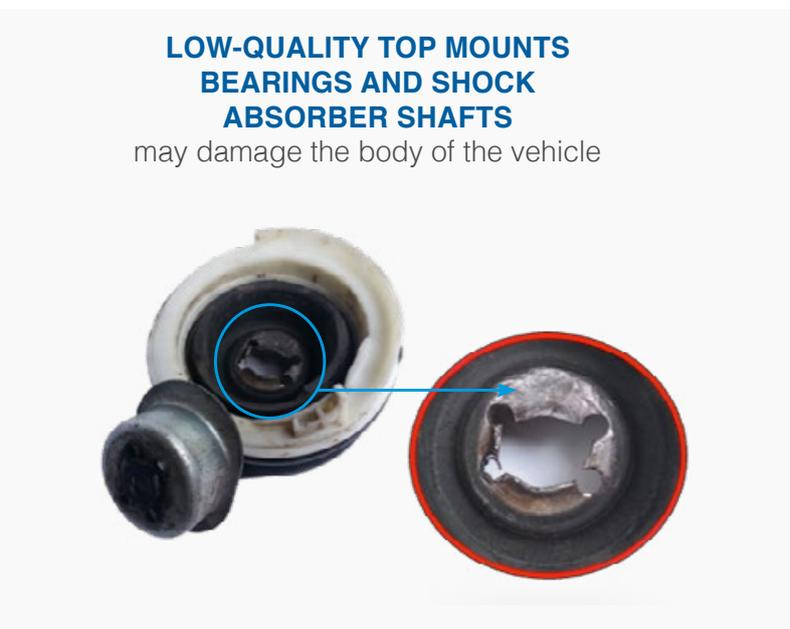
Some brands choose to imitate the shape and colour of a part in order to create the impression that it is comparable to the original equipment part. But since the specifications of the original equipment are not maintained (heat treatment, metal reinforcements...), the use of such products may result in their puncturing the body of the vehicle in the event of impact.
