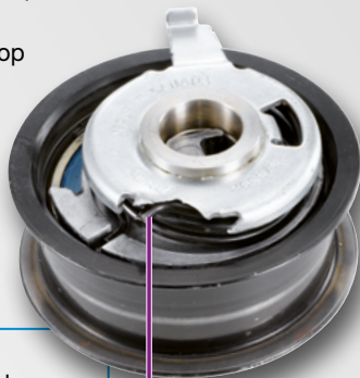
Lower stop marked or broken
