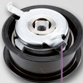
Upper stop marked or broken
