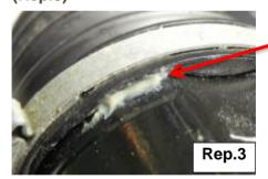
Not enough tightening: Grease leakage
