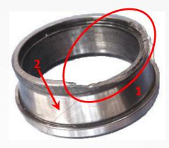
The fragments of the broken collar then find their way into the raceways of the bearing this soon results in noisy bearing and eventually destroys the bearing entirely
