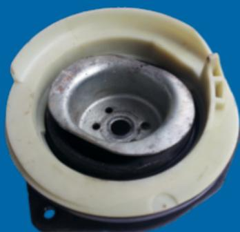
**LOW-QUALITY TOP MOUNTS BEARINGS AND SHOCK ABSORBER SHAFTS** may damage the body of the vehicle
