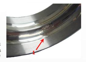
Installing the bearing backwards causes the ABS calculator to malfunction (error code, ABS warning lamp). The bearing cannot be removed and refitted. When installing the bearing, make sure that the side with the magnetic encoder is fitted facing the interior of the vehicle (i.e. facing engine / gearbox).
