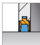
Felt strip seal Well suited for higher rotational shaft speed
