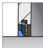
V-Ring seal Reduced friction
