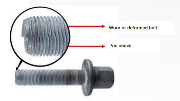
Once a stretch bolt is used the mechanical characteristics of the bolt are changed, the bolt is no longer within the manufacturers specified tolerance's.
