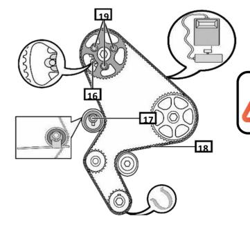
The crankshaft and the injection pump gear must not be rotated while the timing belt is removed.
