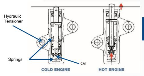
Pressure applied by the hydraulic damper when the engine works at high temperature
