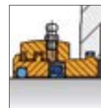
Taconite seal Multiple seal for harsh environments
