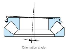
Lubrication: thrust spherical roller bearings are usually heavily loaded and must be lubricated with oil. Due to the internal construction of these bearings, grease lubrication is only possible at low speeds and with limited loads.
