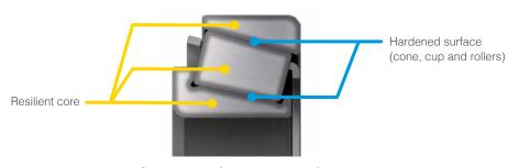
Cross-section of a bearing made of case hardened steel
