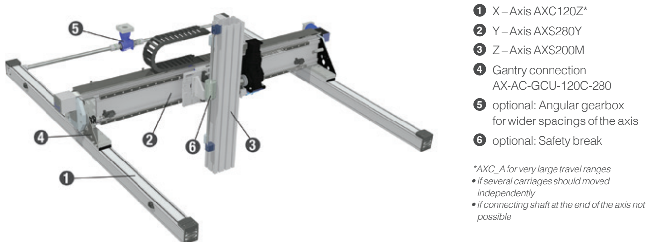
Figure 7.6 — 3-Axis-System AXC120Z(A) – AXS280Y – AXS200M
