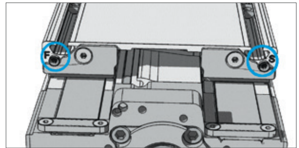
Figure 1.13 — Slider unit with grease nipples on the front side
