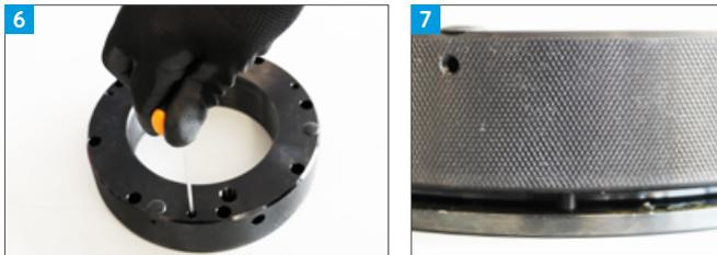
b. Then remove the ejector pins. They are not required during the subsequent operations.
