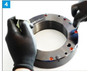
j. Apply thread lock to the compression bolts and screw in so that they are flush with the outside of the piston.
