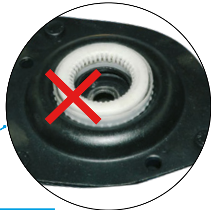
Incorrect installation steering system rotation impaired
