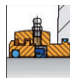
Taconite seal Multiple seal for harsh environments
