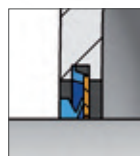
V-Ring seal Reduced friction
