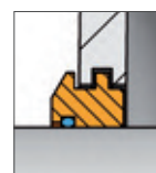
Labyrinth seal Well suited for high temperature applications
