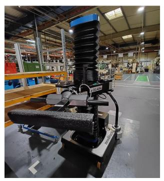
To produce splines, we use rolling machines. These machines are equipped with racks enabling the correct shape to be achieved. The difficulty with these racks is their weight. Each module weighs from 25 kg to just over 30 kg. They need to be changed at the end of each production run, and require regular "re-cutting". To make it easier to fit the racks and ensure better safety for our staff, NTN TE has invested in new handling equipment.
