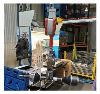
The inspection/packaging zone has also been provided with handling equipment to make operators' work easier and reduce the need to carry heavy loads. Consisting of a standard mobile gantry and a specific gripper developed in-house, the system meets the needs of our staff. Given the success of this prototype and the positive feedback, the solution will be duplicated at the three other workstations in this zone.
