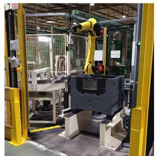
An initial robotic unit entered operation during 2023. This removed the need to carry parts at the beginning of one of our ball joint turning lines. The first unit has given complete satisfaction to operators and the maintenance teams. As a result, the decision was taken to duplicate and adapt this unit to another turning line. The second unit entered service in 2024 with a slightly different technology. The first is a bin picking
