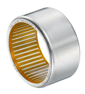
Bearings with solid grease resist grease leakage even in applications where strong vibrations, centrifugal force, moisture, etc. are present, eliminating greasing and installation of greasing nipples. It eliminates the need to grease the bearings when assembling therefore, the installation of grease nipples is not required. As it retains the rollers in position during assembly, the rollers do not drop during assembling, making it easier to handle the bearings.
