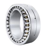
Thanks to its ductility, brass also allows for preventive maintenance. In the event of an advanced state of wear of a bearing, a brass cage will not break suddenly, rather will emit a specific sound, indicating it will soon need to be replaced. Potentially severe collateral damage linked to the failure of a bearing can thus be prevented. The shaft and housings can for example be damaged and entail costs that are much higher than that of the mere replacement of the bearing.
