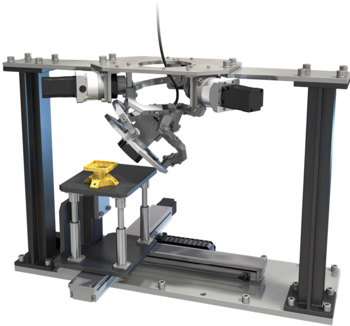
Le robot parallel link PHACE
